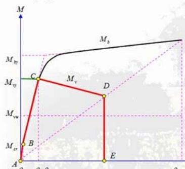
(b) Flexure-Shear failure
