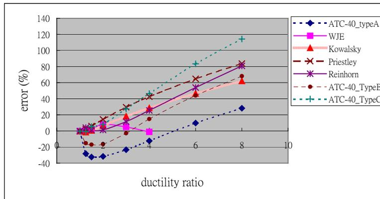
Fig. 5 Error in the estimated displacement response characterized by that in  $SR_{AD}$
