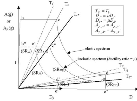
Fig. 2 Equivalent elastic and inelastic design diagram
