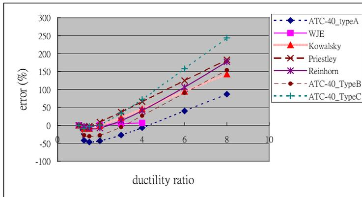
Fig. 4 Error in the estimated displacement response characterized by that in  $SR_{VD}^2$
