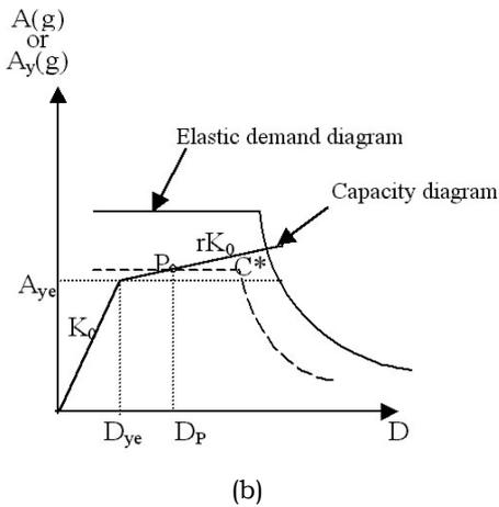
Fig. 3 Performance point from a non-iterative capacity-spectrum method
