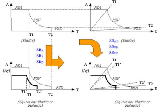
Fig. 1 Spectrum and diagram reduction factors
