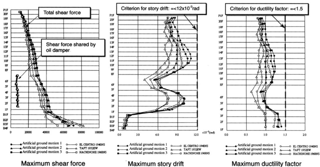
Fig. 23 Maximum floor responses (X-direction)
