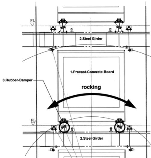
Fig. 32 Outline of structural control device using high-damping rubber
