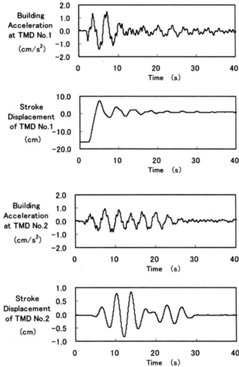
Fig. 28 Responses obtained from free vibration test
