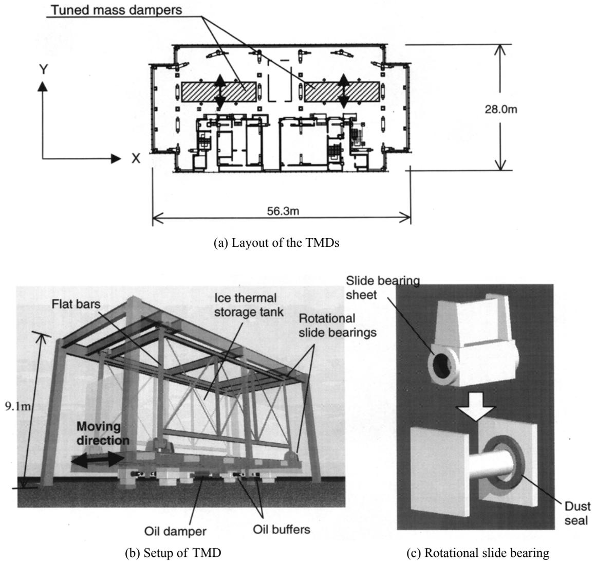
Fig. 25 Layout and setup of TMD and slide bearing
