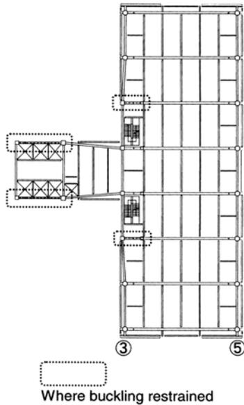
Fig. 17 Framing plan of typical floors
