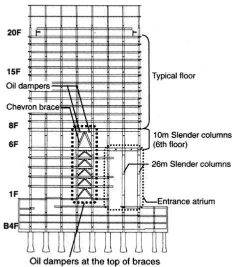
Fig. 18 Building elevation of Building B
