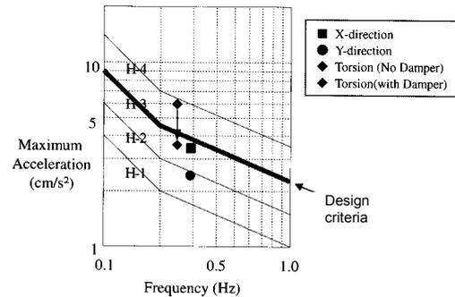
Fig. 33 Effect of structural control on reduction of vibration
