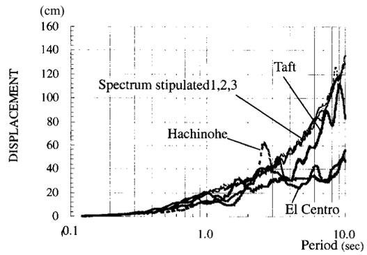
Fig. 10 Displacement response spectra (5% damping)
