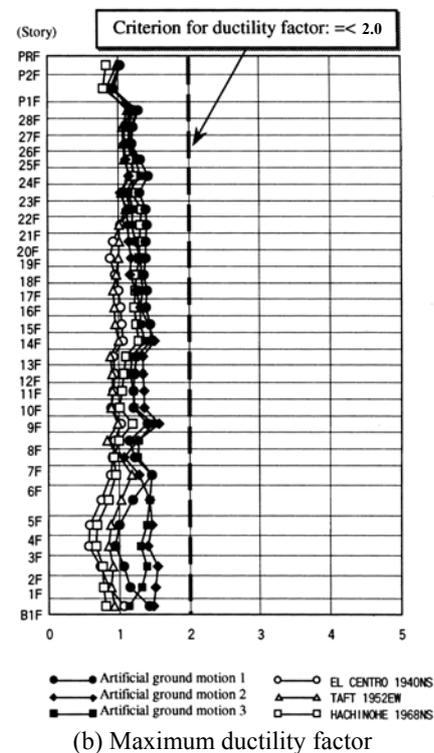
Fig. 13 Maximum responses of main frame (X-direction)
