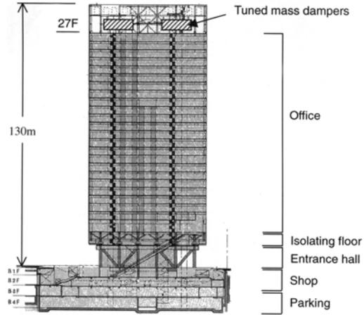
Fig. 24 Vertical section of Building C
