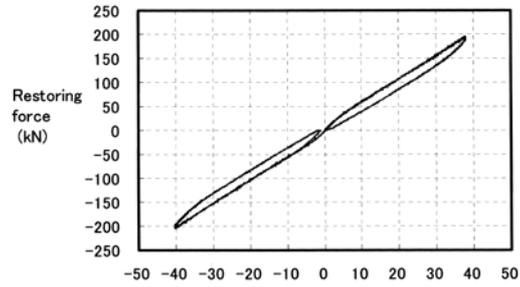
Fig. 27 Force-displacement loops of slide bearing
