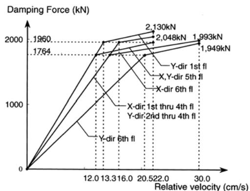
Fig. 20 Force-velocity relationships of oil dampers
