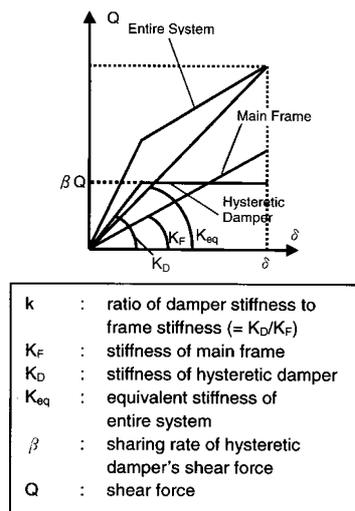
Fig. 7 Typical hysteresis characteristics of building with steel hysteretic dampers
