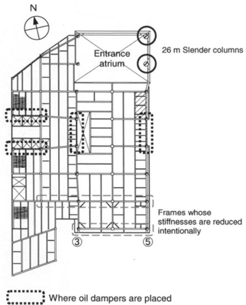
Fig. 16 Framing plan of lower (3rd) floor
