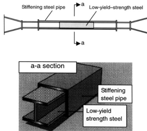
Fig. 5 Outline of buckling restrained brace
