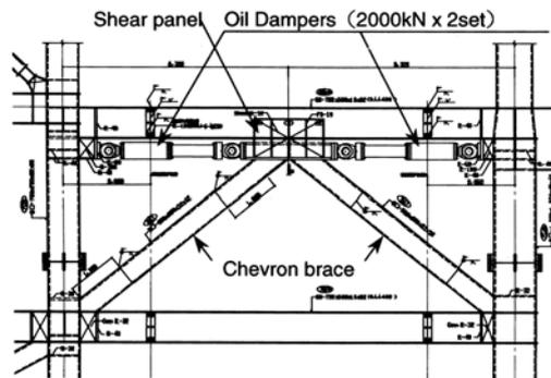
Fig. 19 Oil dampers installed in frame
