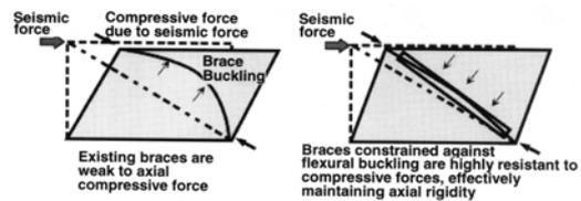
Fig. 4 Deformation of existing brace and brace constrained against flexural buckling
