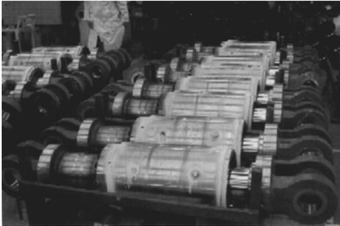
Fig. 21(a) Oil dampers in manufacture
