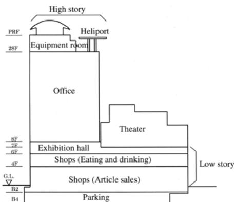
Fig. 2 Sectional layout of Building A
