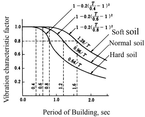
Fig. 1 Vibration characteristic factor  $R_t(T)$
