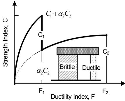
Fig. 2 Force-deformation relation of two-member system
